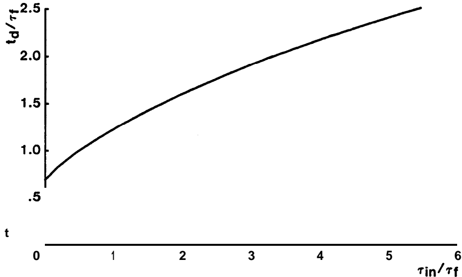
Figure 5.7 Gate delay for an exponential input.
