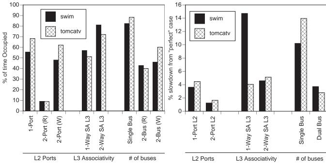
**Figure 3:** Resource occupancies in Hydra for several simulated situations. (see section 3 for the L2/L3 cache discussion and section 4 for discussion of the buses)
