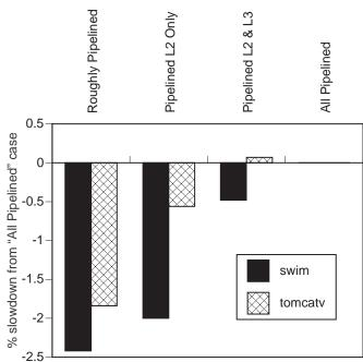
**Figure 5:** The % increase in execution time, over "perfect" scenarios with no arbitration at all between fully pipelined state machines, seen as a result of variations in the arbitration mechanisms and pipelining of the read and write control state machines. (see section 5 for discussion)
