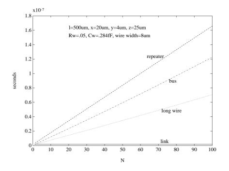
Figure 6.15: Delay versus N, excluding transmission gate
