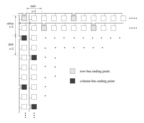
Figure 6.3: Torus with segmented reconfigurable bus, segment length=5, shift=2, offset=2. Only part of the network is shown for simplicity.
