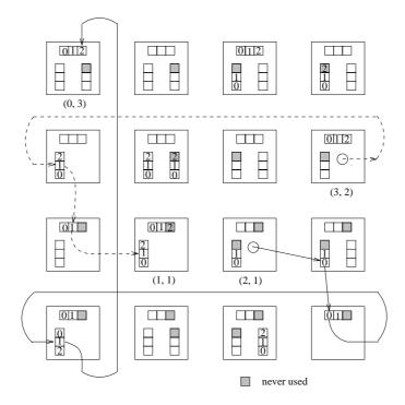
**Figure 4.7**: Examples of Virtual Network routing on the negative network in a 2-D torus. Packets are routed from (2,1) to (0,3) and from (3,2) to (1,1).
