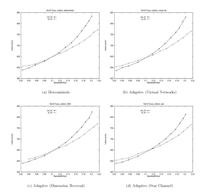
Figure 5.9: Latency versus throughput for different routing algorithms under uniform random traffic. Comparison of uni- and bi-directional channels
