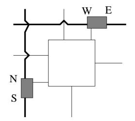
Figure 6.5: A node of the torus with reconfigurable bus.
