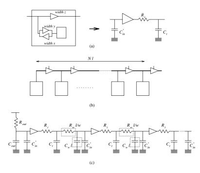
**Figure 6.11:** (a) repeater model, where  $R_t = \frac{40k}{z}$ ,  $C_t = 4z + 10$ ,  $C'_{in} = C_{in} + 2C'_g$ , (b) repeater interconnection, (c) repeater interconnection model
