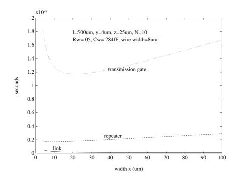
**Figure 6.12**: Delay versus transistor width x for a fixed width z
