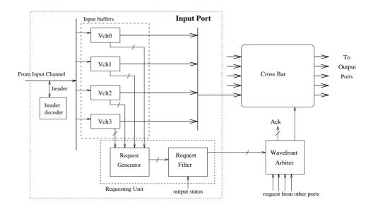
Figure 5.1: Internal router node architecture model
