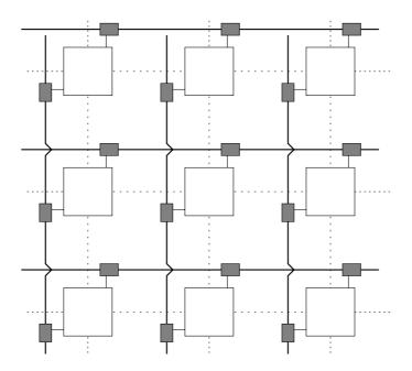
**Figure 6.1**: Torus structure with links and reconfigurable buses. Dotted lines are the links connecting nearest neighbors. Solid lines are the reconfigurable buses. The wrap-around connections of the torus are not shown. Also see Fig. 6.2 for detail connections.
