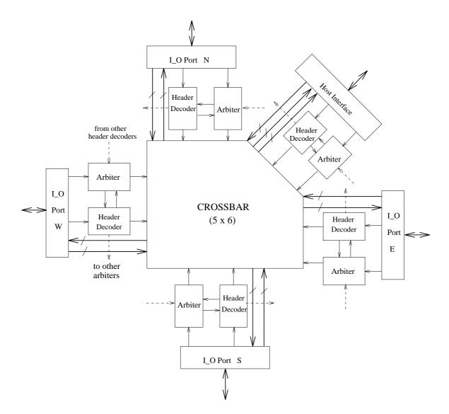
Figure 7.5: Global router architecture
