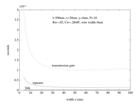
Figure 6.13: Delay versus transistor width z for a fixed width x
