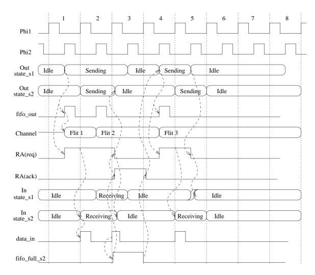
Figure 7.11: I/O control and channel timing diagram
