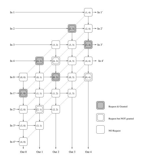
Figure 5.2: Wavefront arbitration. Each cell corresponds to a cross point in the crossbar switch.
