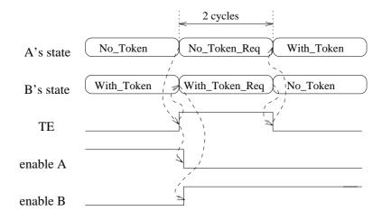
Figure 3.6: Token exchange timing diagram
