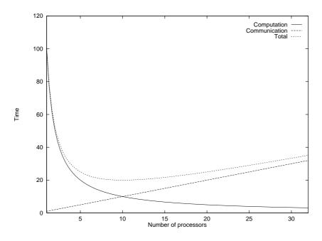
Figure 1.4: Total execution time is composed of computation time and communication time
