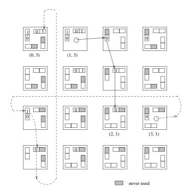
Figure 4.4: Examples of dimension-order routing in a 2-D torus. Only input buffers are shown. Some buffers are omitted for simplicity. Packets are routed from node (3,1) to (0,3) and from (1,3) to (2,1). Half of the upper channels are never used (shaded buffers) because the maximum packet distance is half the torus size due to wrap-around connections.
