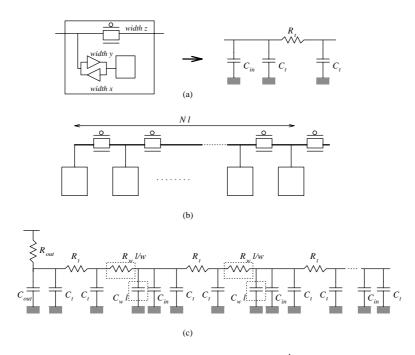
**Figure 6.10**: (a) Transmission gate model, where  $R_t = \frac{40k}{z}$ ,  $C_t = 4z + 10$ , (b) Transmission gate interconnection, (c) Transmission gate interconnection model
