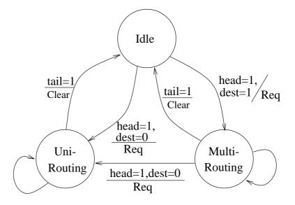
Figure 7.9: State diagram of the header decoder
