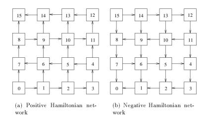
Figure 4.18: Partition of a 2-D mesh based on the Hamiltonian path  $\mathbf{F}$
