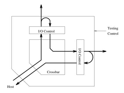
Figure 7.25: Loop-back mode test
