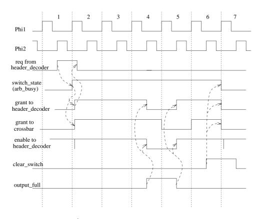
Figure 7.16: Arbiter timing diagram
