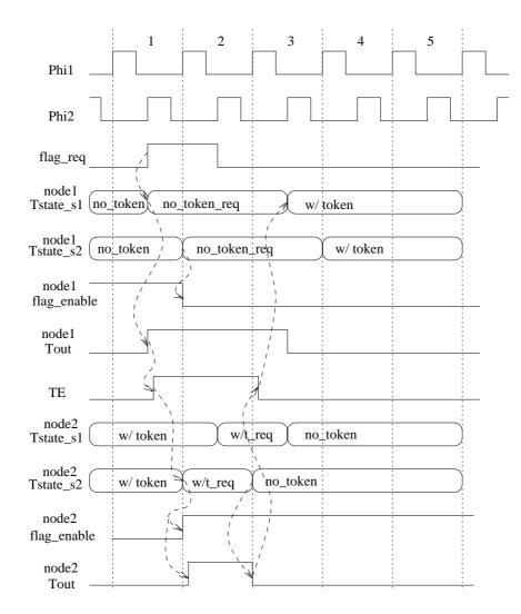
Figure 7.14: Token-exchange timing diagram
