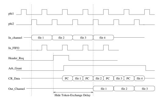
Figure 7.18: Router core timing diagram
