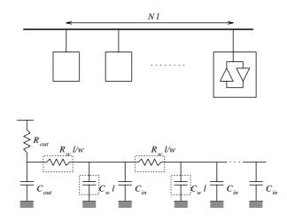
Figure 6.9: Bus model, where the parameters are the same as link model
