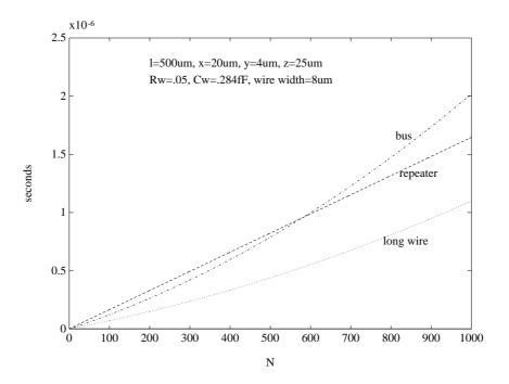
Figure 6.16: Delay versus large N
