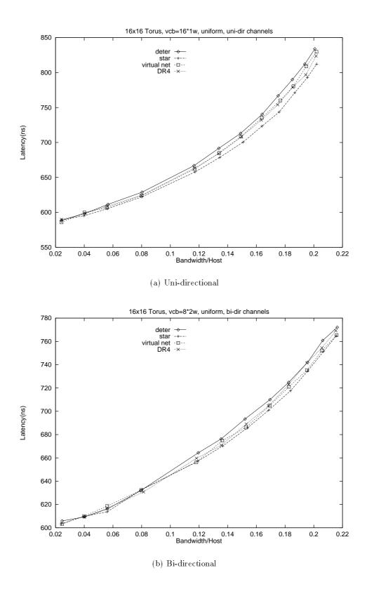
Figure 5.6: Latency versus throughput for different routing algorithms under uniform random traffic
