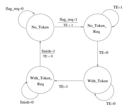
Figure 3.5: Token exchange state diagram
