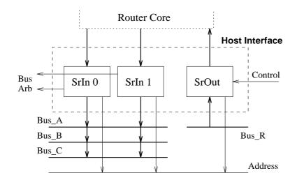
Figure 7.6: Host interface architecture
