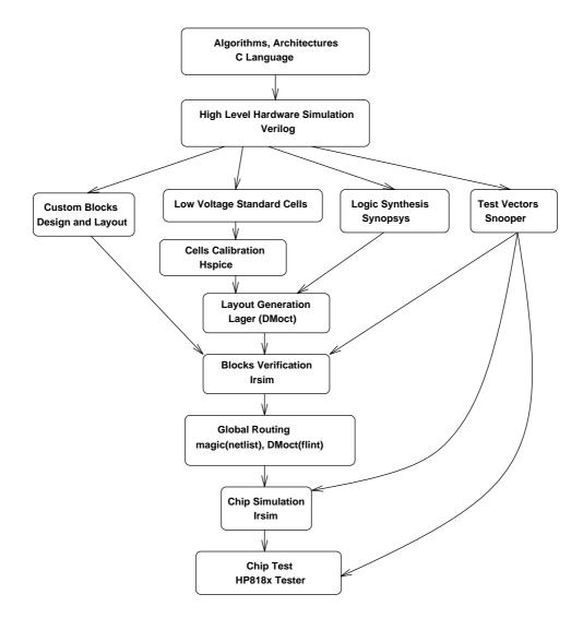
Figure 7.19: Design methodology and flow of STARP
