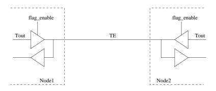
Figure 7.12: Token-exchange interface circuit diagram
