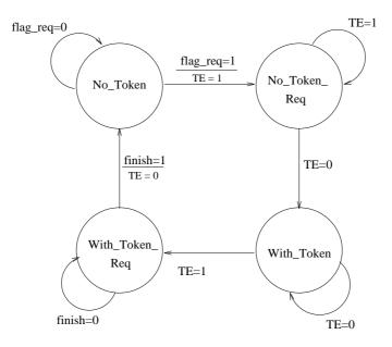
Figure 7.13: Token-exchange state diagram
