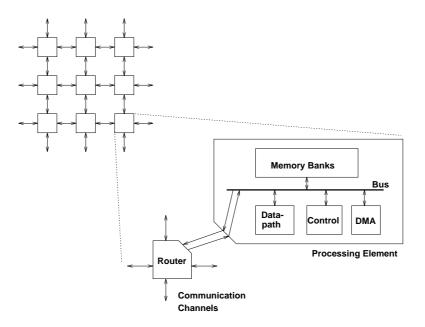
Figure 7.1: Network architecture of STARP
