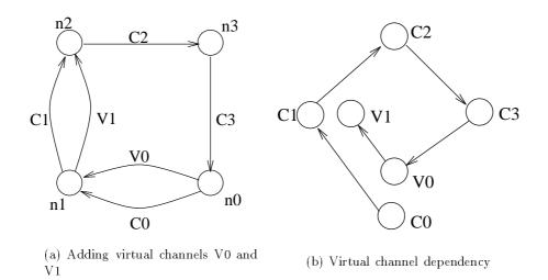
Figure 4.3: Deadlock avoidance by adding virtual channels
