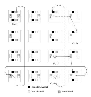
**Figure 4.9:** Examples of Star-Channel routing in a 2-D torus. Packets are routed from (2,0) to (3,2) and from (2,1) to (0,3).
