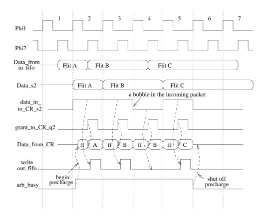
Figure 7.17: Crossbar timing diagram. ff in Data from CR is the precharged value.
