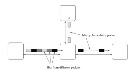
Figure 5.15: Interleaving flits from different packets will insert idle cycles in the packets when they continue to the next node.
