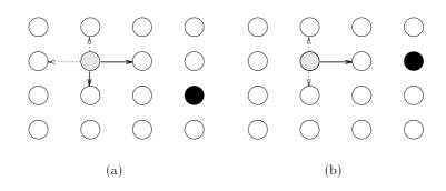
**Figure 4.13**: Derouting in a 2-D array when a packet is blocked. The shadow circle is the current node and the black circle is the packet's destination. Solid lines are the normal paths, and dotted lines are the derouting paths.
