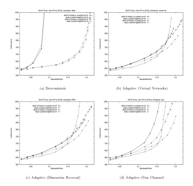
Figure 5.14: Latency versus throughput for different routing algorithms under transpose traffic.
