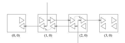
Figure 4.16: Deadlock configuration in tree-based multicasting
