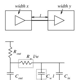
Figure 6.8: Link model, where the wire is modeled by distributed RC
