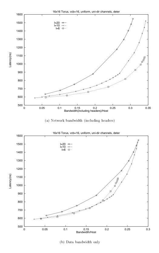
Figure 5.12: Latency for different packet length. Uni-directional channels. Deterministic routing under uniform random traffic.
