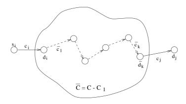
Figure 4.10: Indirect channel dependency from  $c_i$  to  $c_j$ . Solid lines  $\in C_1$ , and dashed lines  $\in \overline{C} = C - C_1$
