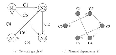
**Figure 4.2**: Relation between network graph G and channel dependency D. The edge between C1 and C2 in channel dependency D indicates that C2 can be used immediately after C1 (via Node N2)
