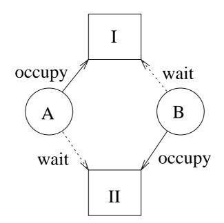
Figure 3.1: An example of deadlock: A is waiting for B to release resource II, and B is waiting for A to release resource I.
