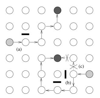
Figure 4.12: Examples of paths for the *negative-first* algorithm of the Turn model in a 2-D mesh
