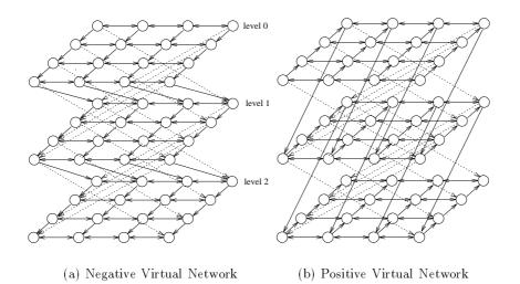
Figure 4.6: Expanding a virtual network to three logical levels in a 2-D torus
