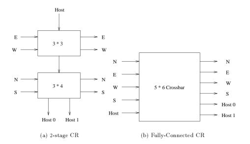
Figure 7.10: Two different crossbar architectures
