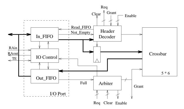
Figure 7.7: Router port architecture, only one port is shown
