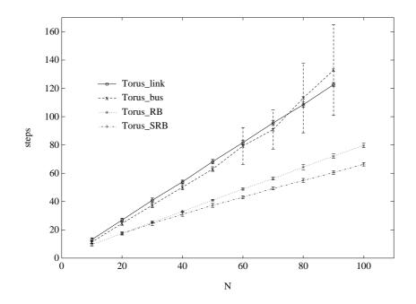
Figure 6.19: Average steps versus N, buffer size=5 for Torus\_link, Torus\_bus, and Torus\_RB, buffer size=10 for Torus\_SRB, segment length=10 for Torus\_SRB
