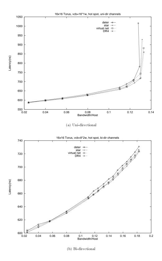
Figure 5.8: Latency versus throughput for different routing algorithms under Hot-spot traffic
