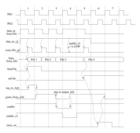
Figure 7.15: Header decoder timing diagram
