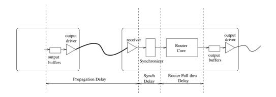
Figure 5.5: Delay components in the simulation model
