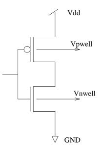
**Figure 7.20**: CMOS inverter model. Vpwell and Vnwell can be biased separately from Vdd and GND to improve the performance at low Vdd
