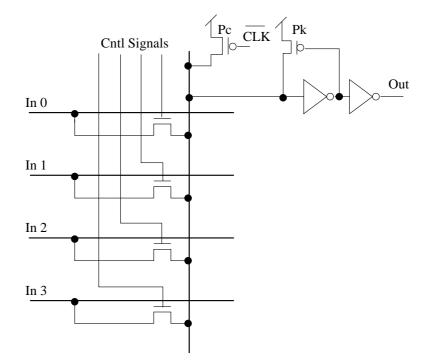
Figure 7.22: Dynamic crossbar switch with a PMOS keeper at the output to prevent leakage
