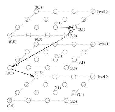
**Figure 4.8:** A packets is routed from (2,1) to (0,3) on the negative virtual network in a 2-D torus. The packet goes to a different logic level when it takes a wrap-around link.
