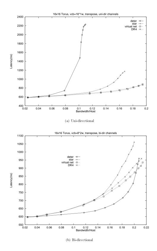
Figure 5.7: Latency versus throughput for different routing algorithms under transpose traffic
