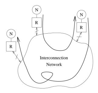
Figure 1.3: Multiprocessor networks. Communication occurs between nodes (processors and/or memory). N is the node and R is the data router.
