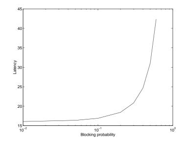
Figure 4.14: Latency penalty due to derouting in a  $16 \times 16$  2-D torus
