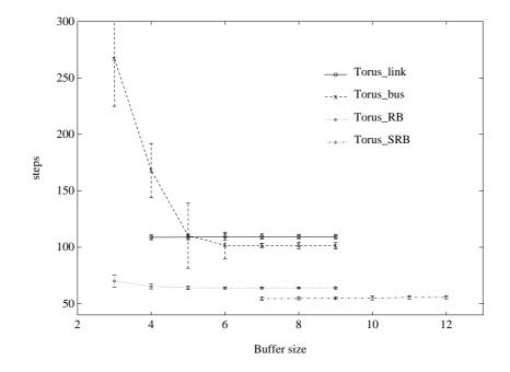
Figure 6.20: Average steps versus buffer size, N = 80, segment length=10 for Torus\_SRB
