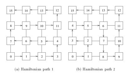
Figure 4.17: Two different mapping to construct Hamiltonian paths in a 2-D mesh
