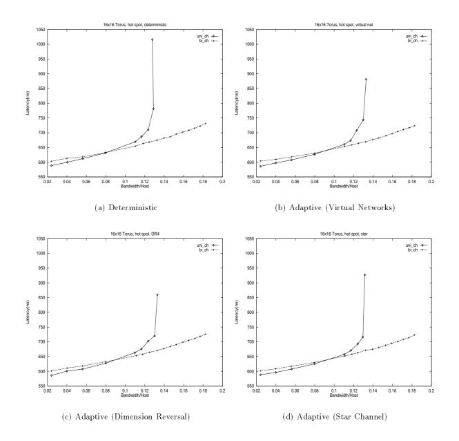
Figure 5.10: Latency versus throughput for different routing algorithms under Hot-spot traffic. Comparison of uni- and bi-directional channels
