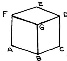
If one knew that this object were lying on the plane determined by ABC which is known, then one would know the projection of each point in the image onto the ABC plane. Each point e.g. F must be on the line determined by its projection onto the ABC plane and the lens center. If the line AF is perpendicular to the plane we then know the length of AF.
