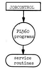
The jobcontrol program and the service routines are executed in the supervisor mode and are storage protected. Together they occupy the first 8000 bytes of core memory.
