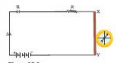
Figure 13.1 Current makes a deflection in position of electric current through a metal conductor.
