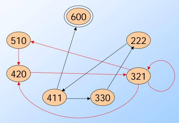
Notice: 600 is a must-fail state; 510, 420, and 321 are can't-fail states; 411, 330, and 222 are "might-fail" states.
