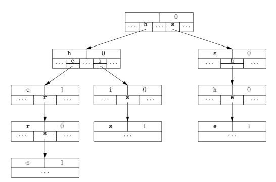
Fig. 5.9. Data structure for the trie of Fig. 5.7.
