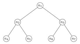
Fig. 5.43. Full binary tree with seven nodes.
